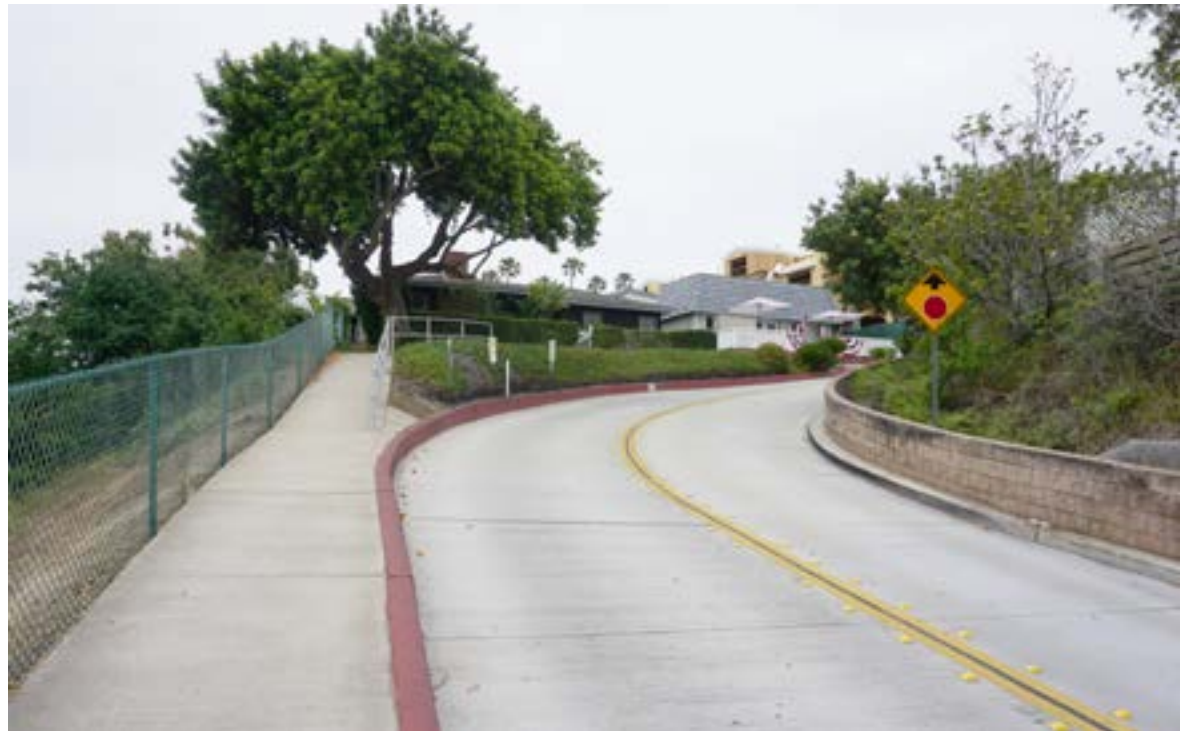
Painted curb to indicate parking prohibited
