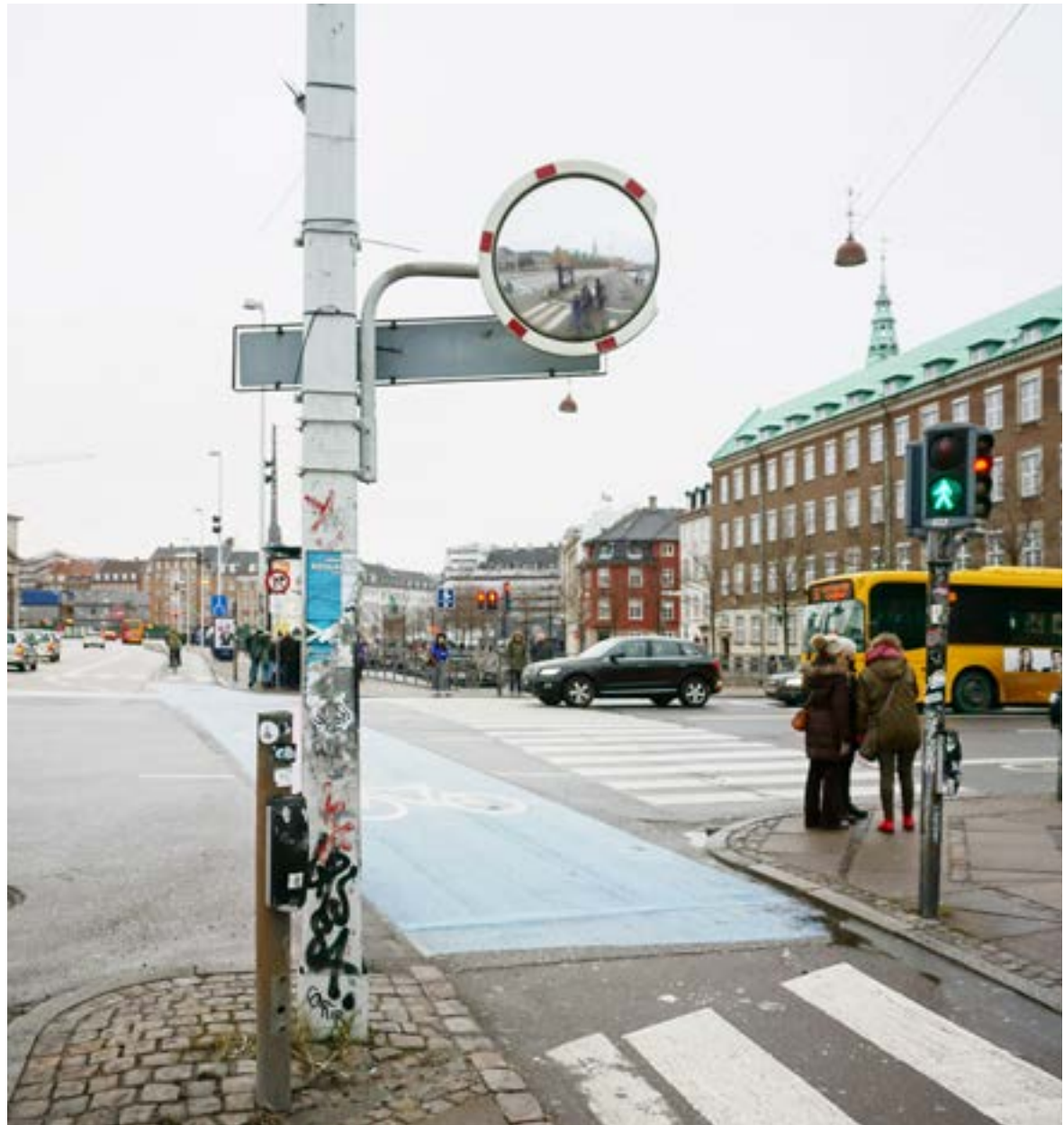
Convex safety mirror mounted to lightpost
