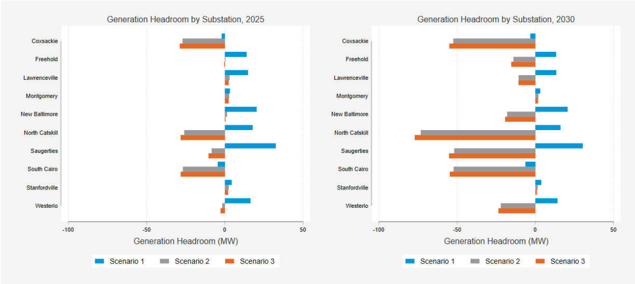
Figure 28: Generation Headroom in MW by Distribution Substation, 2025 and 2030
