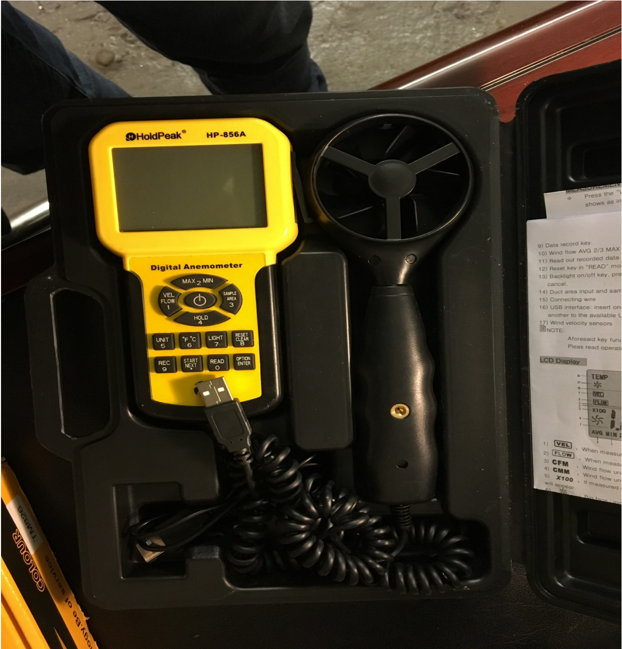
Figure 30. Anemometer for Measuring Cross Section Air Flow
