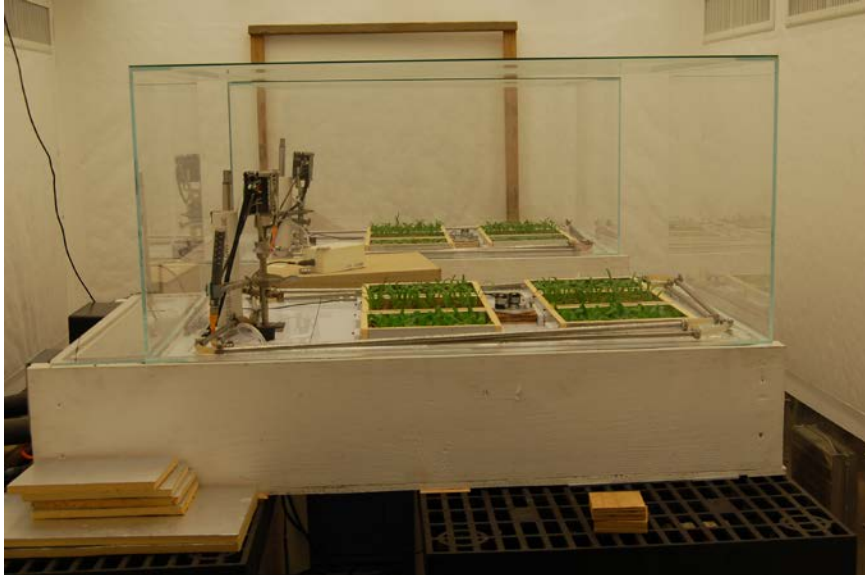
Figure 2. Three crops after thinning, floating in mini-ponds within the mini-chambers, within the walk-in plant growth chamber
