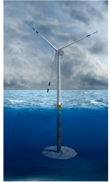
Example of fixed-bottom support
