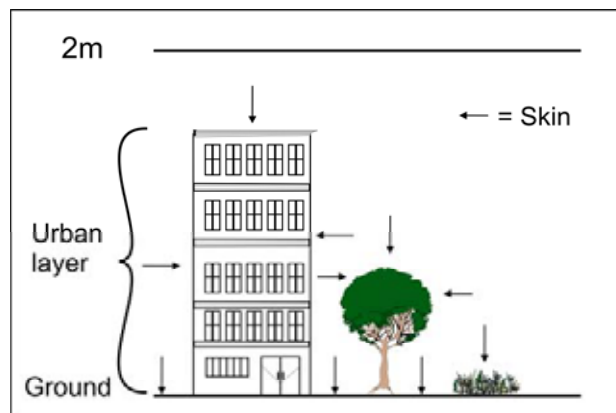
Figure 2-13. Surface (skin) temperature in an urban setting. MM5 sees horizontal surfaces only and the 2-meter temperature is conceptually above city's rooftops.
