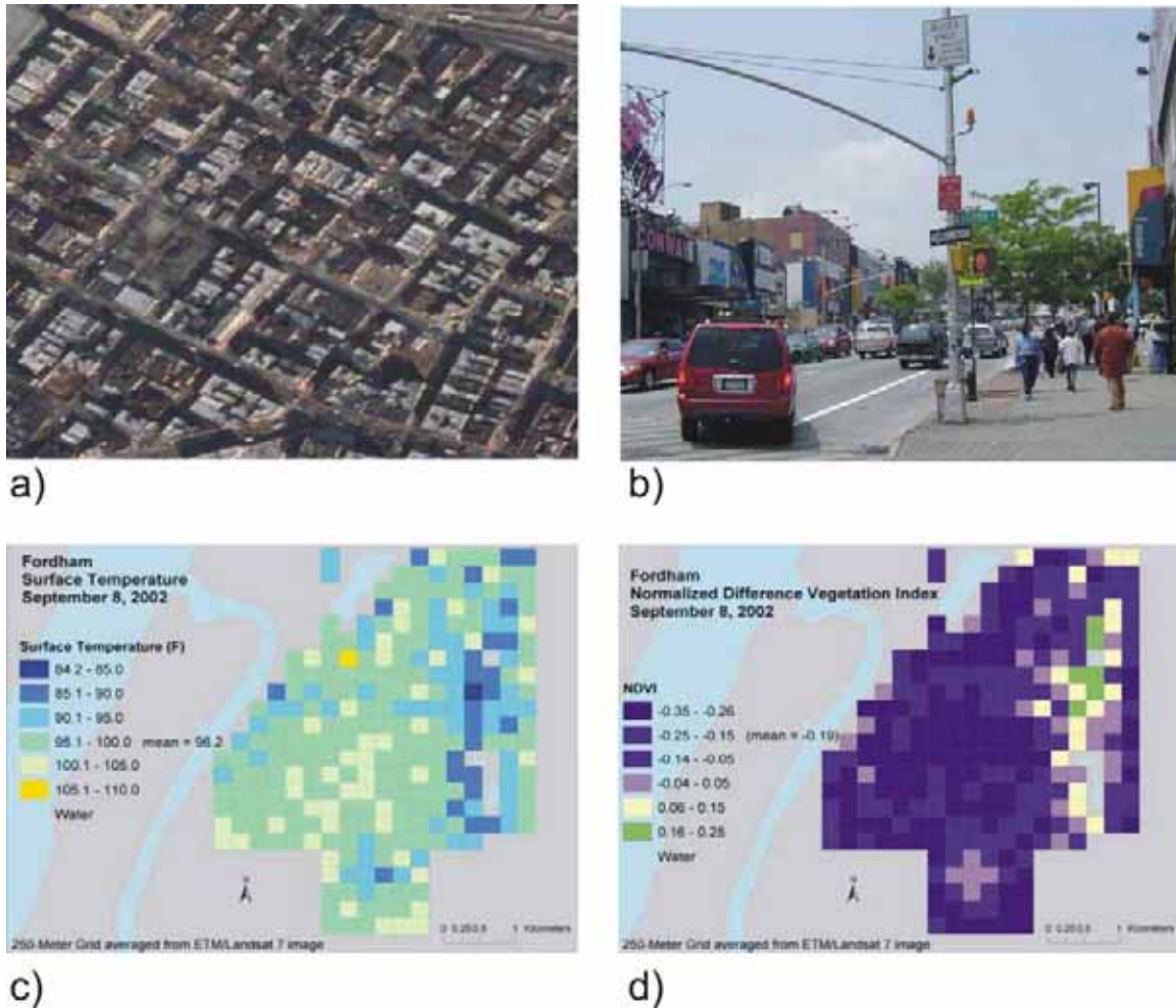
Figure 1-7. Fordham Bronx case study area. a) aerial view, b) street view, c) gridded surface temperature on September 8, 2002 with resolution of 250 meters, d) gridded NDVI with resolution of 250 meters.
