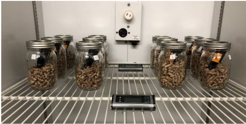
Figure 4. Carbon Monoxide Off-Gassing Experiment in Temperature Controlled Conditions
