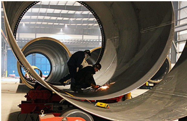
Figure 6. Ventower Welding Tower Sections
