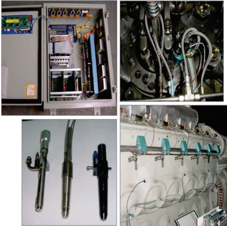
Figure 10. ECI CNG System Components for EMD Locomotives
