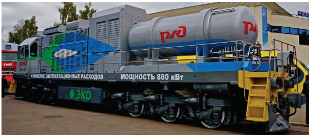
Figure 3. LNG Locomotive Built by Transmashholding for Russian Railways
