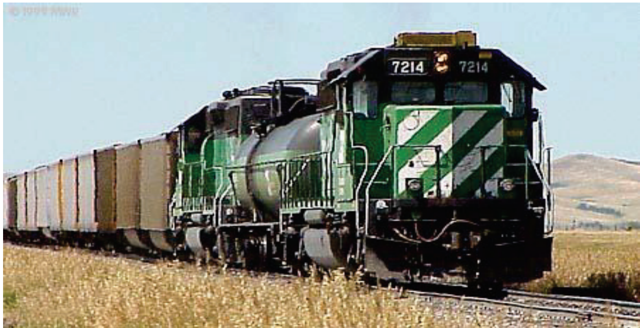
Figure 4. BNSF Test Locomotives and LNG Fuel Tender
