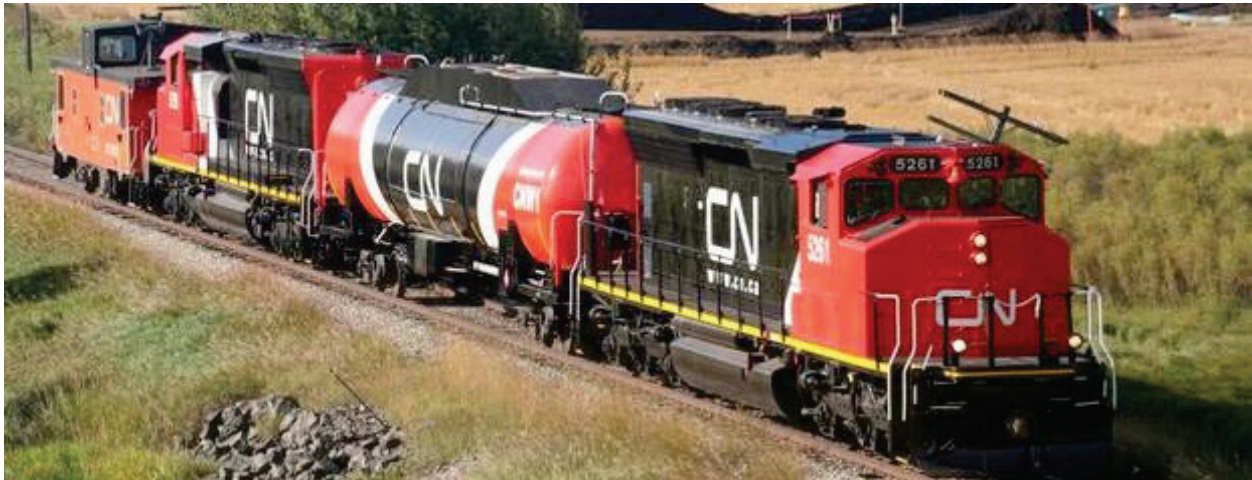
Figure 1. CN Railroad's Test LNG Locomotives and Fuel Tender
