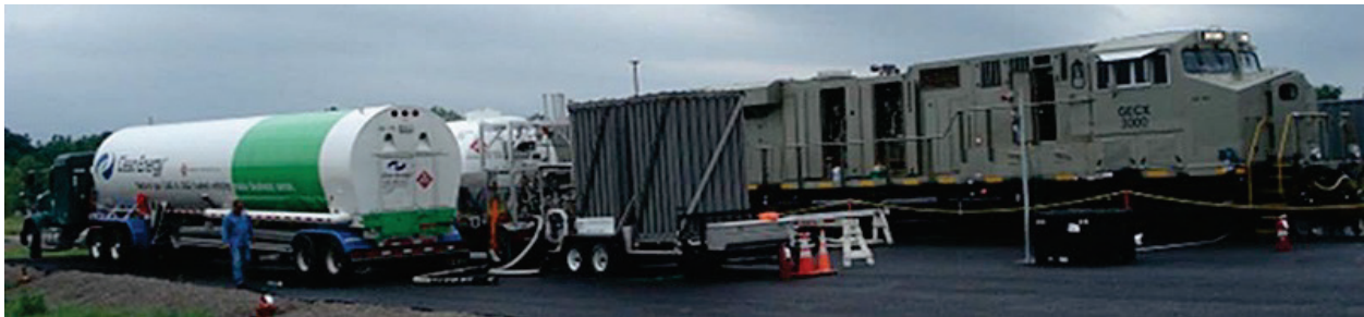
Figure 2. A CSE Operated GE Locomotive being fueled
