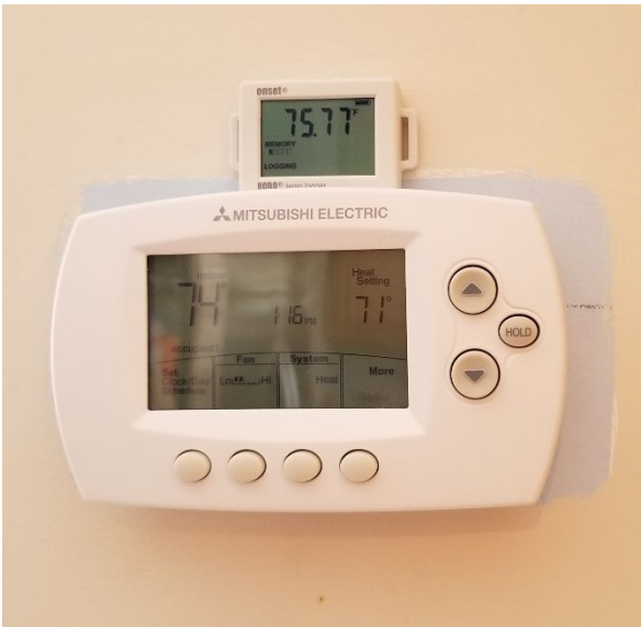
Temperature Data Logger in Living Room
