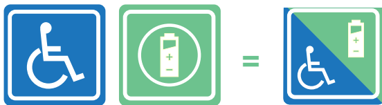
FIGURE 8. MULTI-DIMENSIONS OF ACCESSIBILITY VERTICAL SIGNAGE (SEE SECTION ON SIGNAGE AND WAYFINDING FOR MORE DETAIL) SHOULD DESIGNATE WHETHER EVSE IS WHEELCHAIR- ACCESSIBLE. THE GROUND SURFACE SHOULD BE FIRM, LEVEL, AND HAVE A SLOPE NO MORE THAN 2% IN ANY DIRECTION
