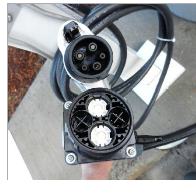
CHAdeMO connector (below) and J1772 connector (above)
