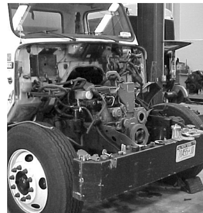
Figure 21. John Deere compressed natural gas engine used to repower Manhattan Beer delivery trucks
