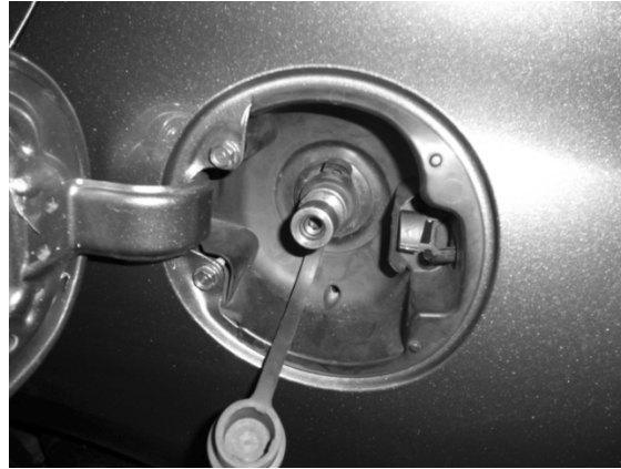
Figure 5. P36 CT1000 compressed natural gas receptacle
