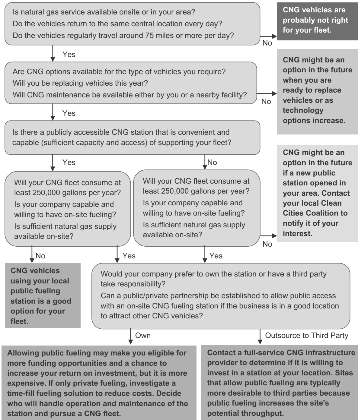
Figure 2. Decision flowchart to determine if compressed natural gas is right for your fleet
