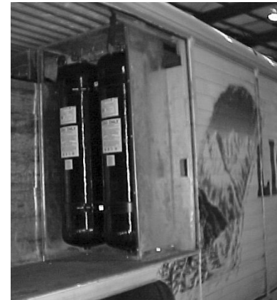
Figure 22. Compressed natural gas tanks installed on Manhattan beer trucks
